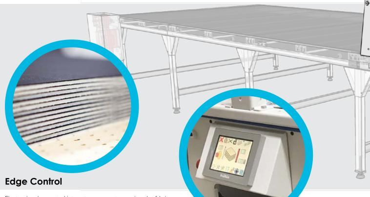
Electronic edge control integrates sensors to monitor the fabric selvedge ensuring that each layer is accurately positioned. A manual override function is included for difficult materials.
